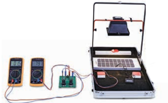
How power output from solar modules depends on temperature
