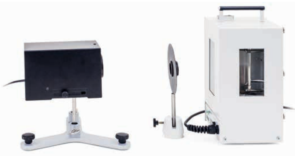
Experiment set-up for transmissive illumination of sodium fluorescence tube with a beam of white light
