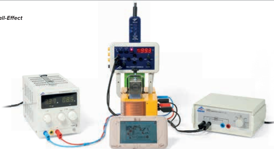
Hall voltage in p- and n-doped germanium as a function of the temperature T
