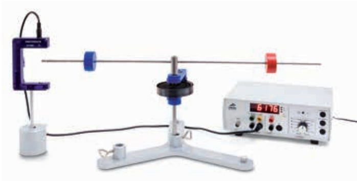
Moment of inertia J of weights as a function of their radius r from the axis of rotation
