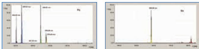
Line spectra of Hg (high-pressure) and Na, recorded using the digital spectrometer
