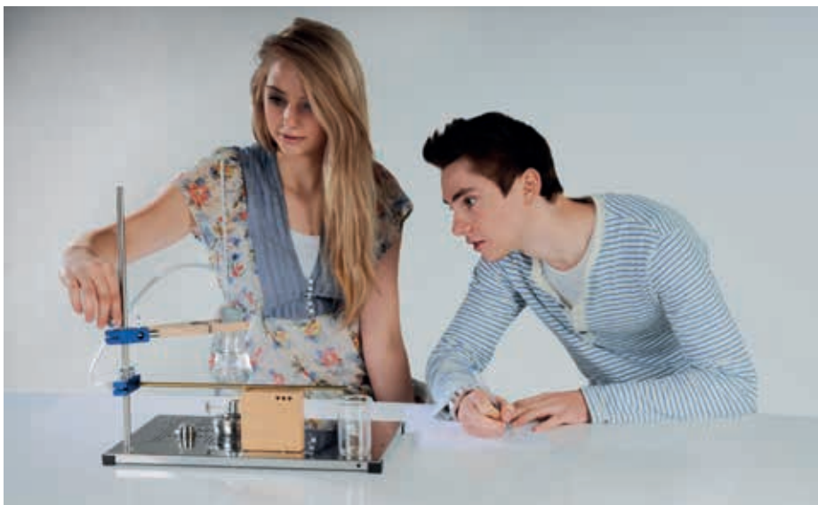
Changes in the length of solid bodies when heated
