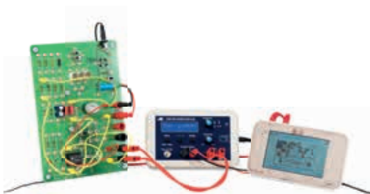
Measurement of a resonance curve for an RLC series resonant circuit
