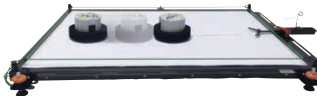
Sample experiment: Elastic collisions
