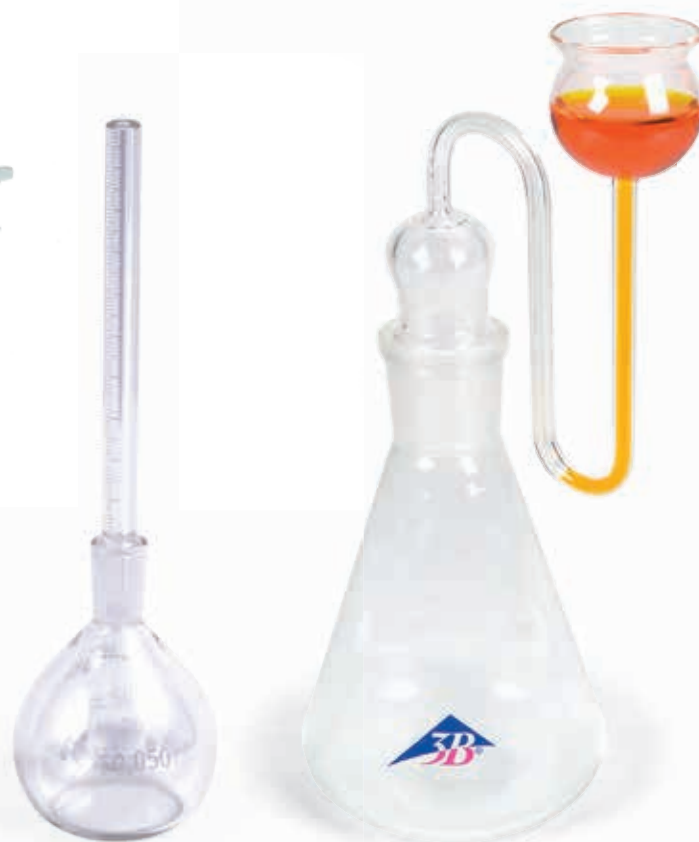
Determining the maximum density of water
