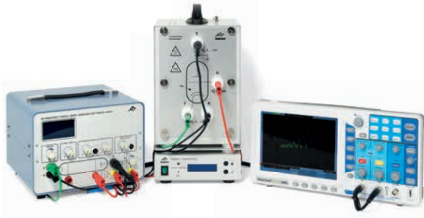
Franck-Hertz experiment with neon
